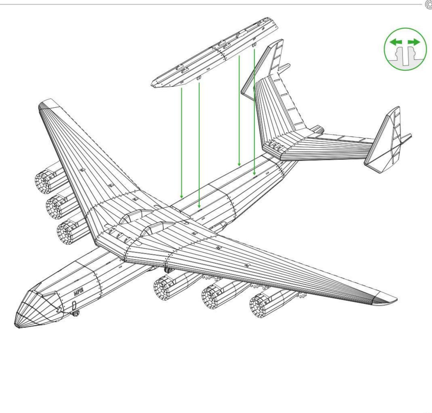
This step uses self-locking lugs that do not require additional fixation. For more reliable fastening, it is recommended to slightly open the fasteners before installation.
